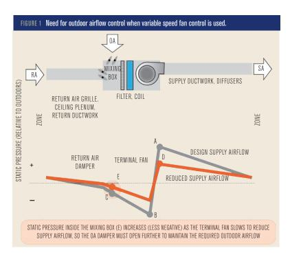
Also, note that these are minimum position setpoints. If the terminal unit includes an airside economizer, the OA damper may be opened further when conditions are suitable for economizer cooling.
