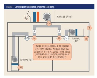
dampers could be used to implement demand-controlled ventilation and reduce outdoor airflow delivered to a zone during periods of reduced population.
